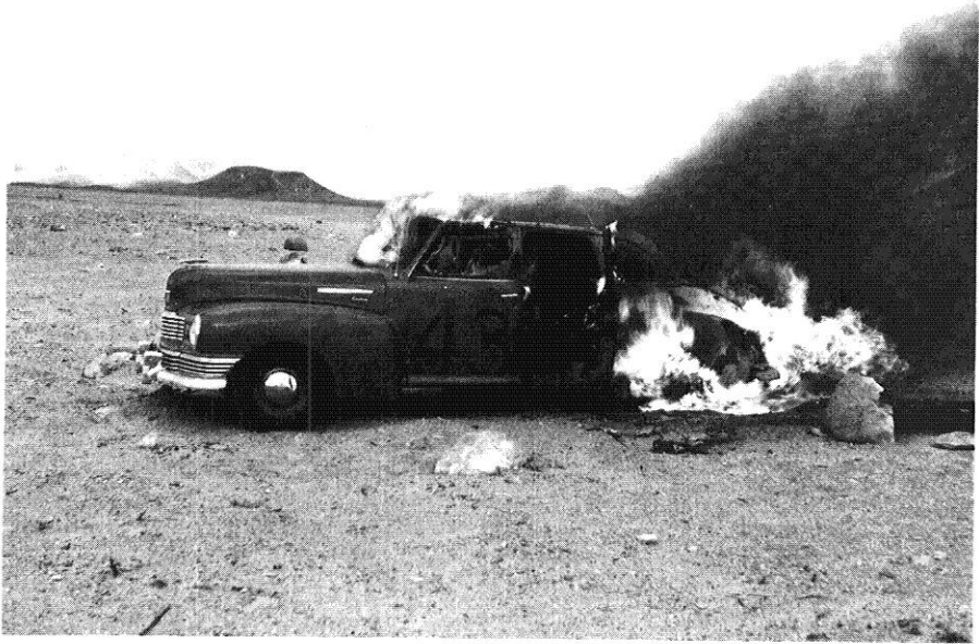
Figure 7.27. Thermal radiation from a nuclear explosion ignited the upholstery and caused fire to spread in an automobile, Nevada Test Site.
