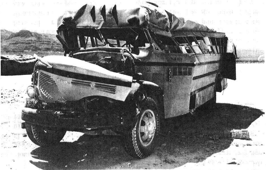
Figure 5.87b. Typical public bus damaged by a nuclear explosion, Nevada Test Site; this bus, like the one in the left background, was overturned, coming to rest as shown after a displacement of 50 feet.
