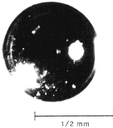
Figure 9.50b. A fallout particle from a tower shot in Nevada. The particle is spherical with a brilliant, glossy surface.
